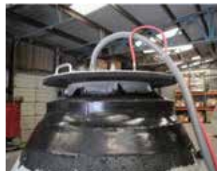
RISER-WRAP® VACUUM TEST
