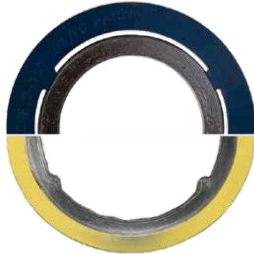
Standard spiral wound gasket shows excessive inward buckling
