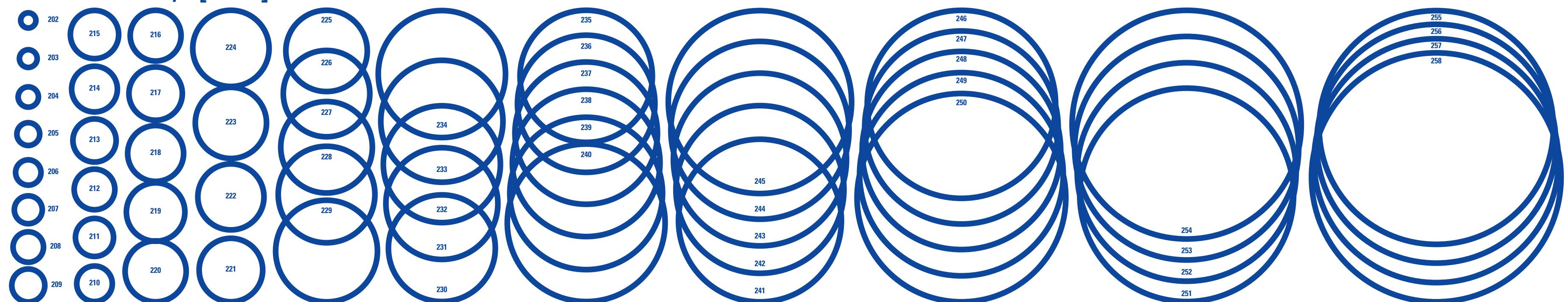
**300 Series 3/16 [0.210] Cross Section 400 Series 1/4 [0.275] Cross Section**
