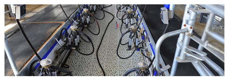
The new and improved Golden Bridge hose support system has a new two piece design made with an impact and abrasion resistant thermo plastic, making it light weight, yet strong as ever.
