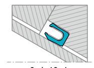
**Conical Seal** Variseal<sup>®</sup> produced in conical arrangement to seal against angled faces.
