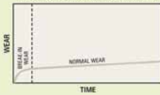
Figure A Typical Wear Behavior For Composite Bearings
