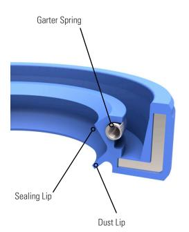
BABSL high pressure rotary seals, available in metric and imperial sizes to suit a wide variety of applications. Pressure resistant style for use without back-up ring, dust lip to protect against outside contaminants, rated up to 10 Bar (depending on other operating conditions).
