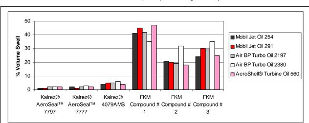
Long-Term Volume Swell In Standard\* & HTS\*\* Gas Turbine Engine Lubricating Oils<sup>1</sup> 1008 Hours at 232°C (450°F) - Oil Changed Weekly<sup>2</sup>
