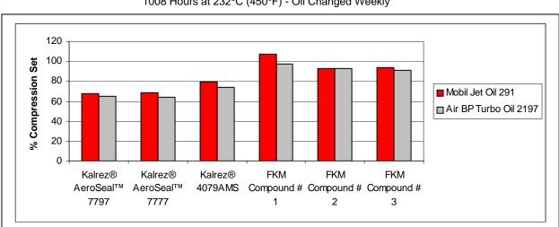
Long-Term Compression Set In HTS\* Gas Turbine Engine Lubricating Oils<sup>1</sup> 1008 Hours at 232°C (450°F) - Oil Changed Weekly<sup>2</sup>
