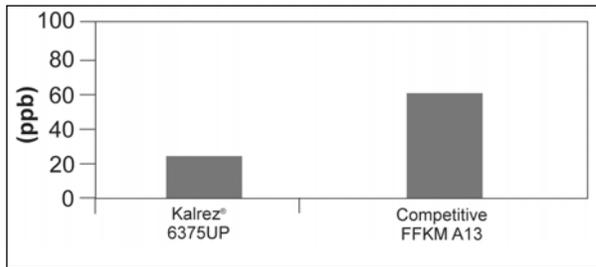
**Total Oxidizable Carbon After Immersion in UPDI Water for 1 Month at 85°C\***
